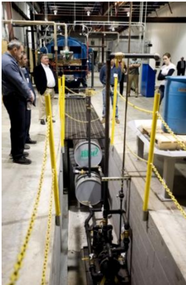
A tour was given of a new venture called RDH Environmental Services located in Cleveland. RDH Environmental takes old tires and recapping materials and through heating process extracts Fuel oil, gas, carbon and sometime steel (if steel was used in the tire). The company says that 1,000 pounds of tires can be processed into 51 gallons of fuel oil, 120 pounds of gas, 200 lbs of steel and 330 lbs of carbon. The process saves landfill space and the recovered material can be used elsewhere. Photo by Jon C. Lakey, Salisbury Post.
