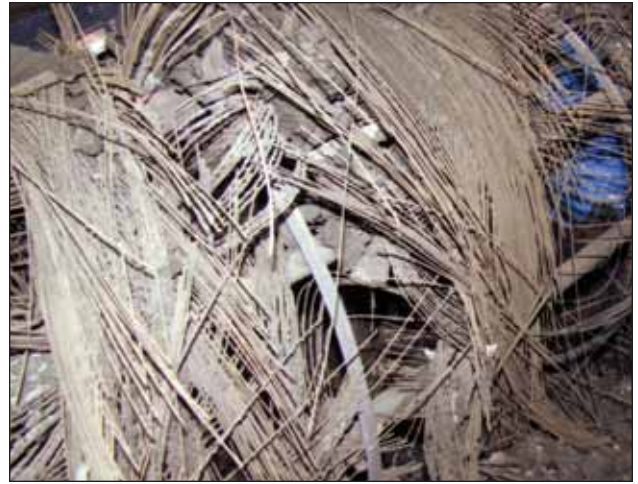
Three 235R25 scrap tires after processing.
